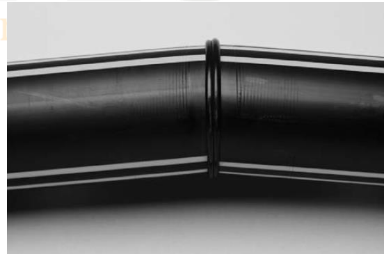
Improper alignment in fusion machine—mitered joint.
