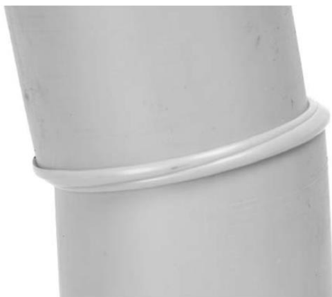
“high-low” pipe alignment. Visually mitered joint.
