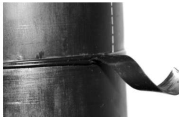
Improper alignment in fusion machine—mitered joint.
