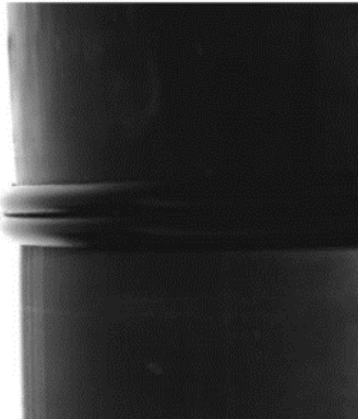
Proper double roll-back bead. Proper alignment.
