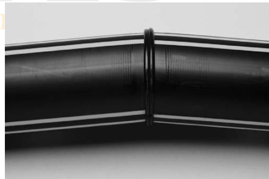
Improper alignment in fusion machine—mitered joint.
