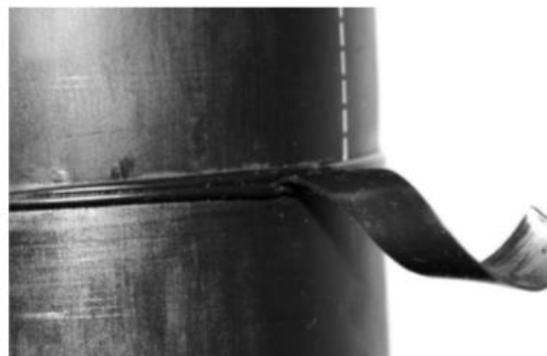
Improper alignment in fusion machine—mitered joint.
